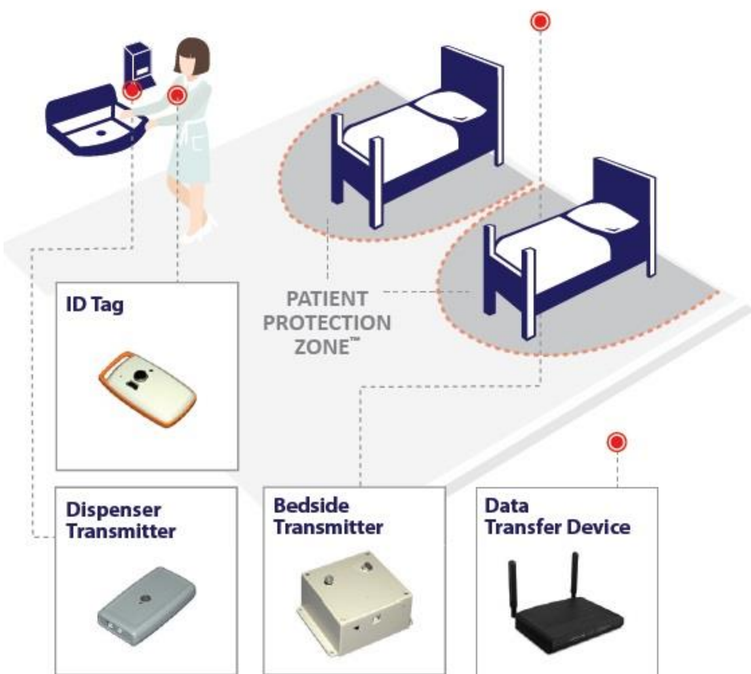
Figure 1. Set up electronic hand hygiene monitoring system
